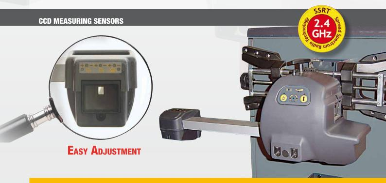
The measuring sensors use the CCD measuring system, and are fitted with 8 sensors for detecting the outer angle edge, the additional measurements, and the real thrust axis of the vehicle. The measuring sensors are electronically levelled.
