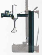
8-11120032 BPL HELP DEVICE Adjustable in height, it is limited to the tyre bead pressure phase from above
